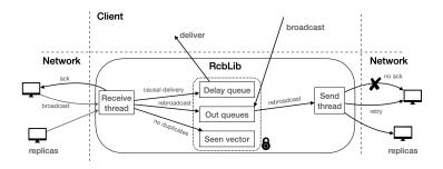
Fig. 3. Structure of the reliable causal broadcast library
